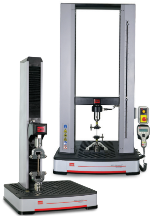
MTS Criterion® Electromechanical Universal Test Systems
