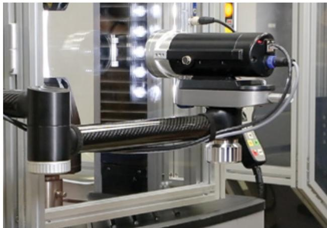
Each AVX Measurement Head includes an inspected, traceable validation block, which can be used to confirm calibration at the beginning a series of tests. Validation blocks are serialized and include an ISO 17025 Accreditation Calibration Report.
