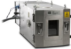
To ensure accurate and consistent results, the MTS 651.05F-01 Environmental Chamber has been tested in DMA applications. It is designed to maintain a constant temperature with very little temperature gradient across the specimen. Heating is achieved with electrical heating elements and a motor-driven fan for diffused convection heat. Cooling is accomplished with liquid nitrogen. It also has a built-in temperature controller, all-welded construction, and Fiberglas™ insulation.
