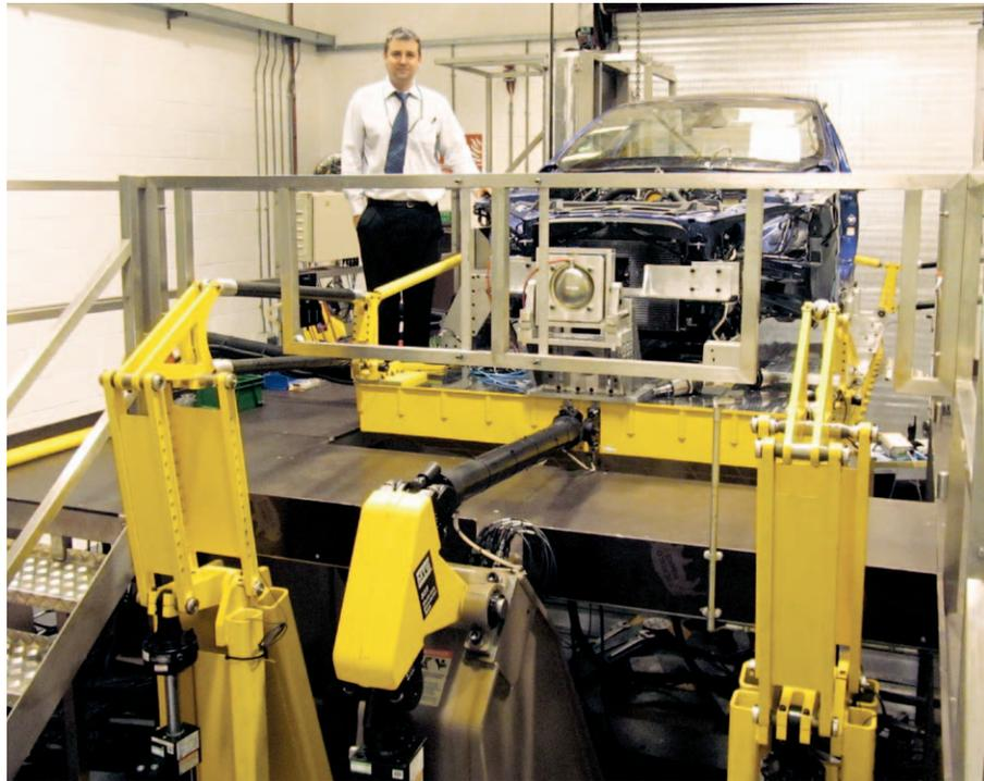
“We're trying to roll as many tests as we can into a single physical prototype,” Payne said. “It's more complex, but we're actually saving a great deal of time during development. The test is also more robust because the system interactions are all working together, which is a lot more realistic.”
