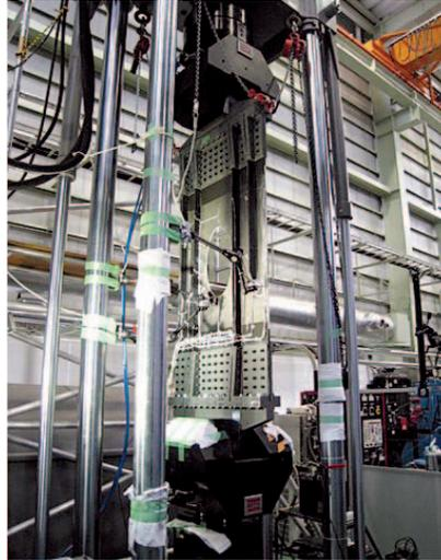
Composite subcomponent fatigue test
