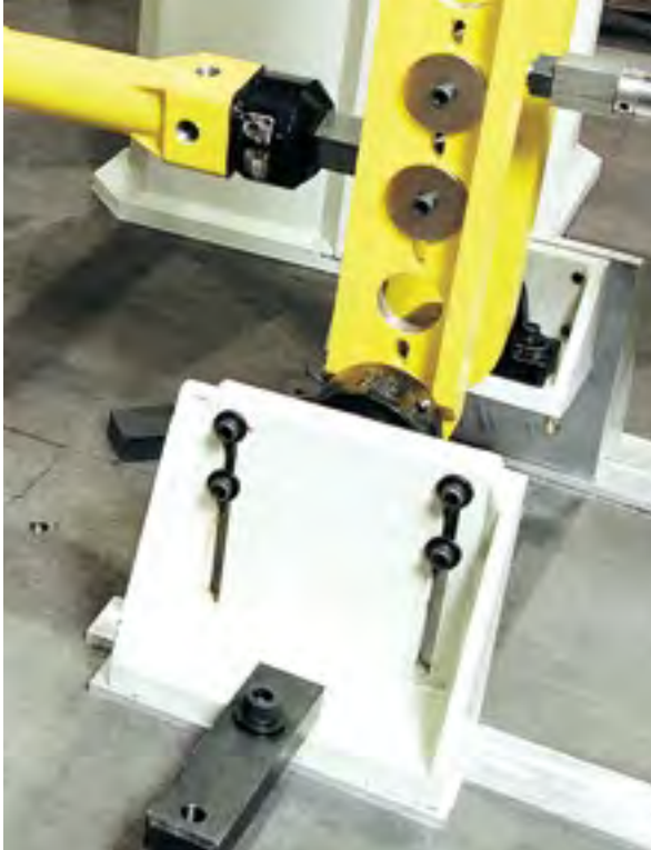
Mounting bracket for levers and bell cranks
