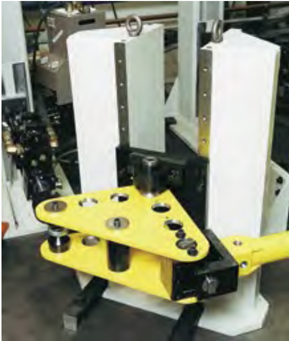
Reaction stands shown with a bell crank
