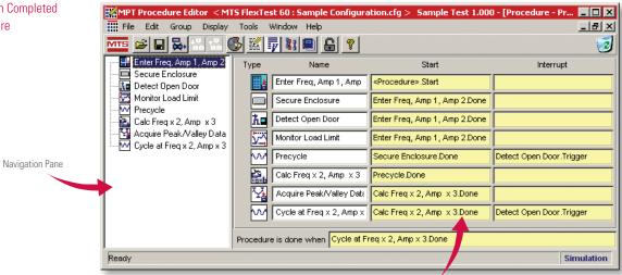
Start and interrupt triggers allow you to direct test flow with precision. To create parallel test branches, you simply assign the same triggers to two or more processes. To end an active process prematurely, you assign an interrupt trigger.
