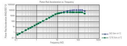
The MTS Model 217 spinning actuator provides highly accurate and repeatable performance in a wide range of frequencies. Note: These are laboratory test results. Real-world capability in a test setup is dependent on the stiffness of the system and specimen.
