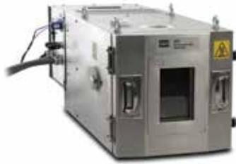
The MTS 651.05 Chamber has been tested in DMA applications. It maintains a consistent temperature gradient across the specimen. It has electrical heating elements and a motor-driven fan for diffused convection heat. Cooling is accomplished with liquid nitrogen.
