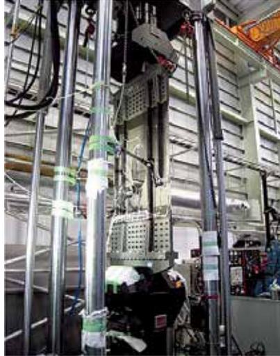
Composite subcomponent fatigue test
