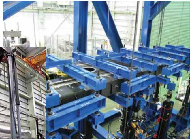
Full-scale composite wing static test
