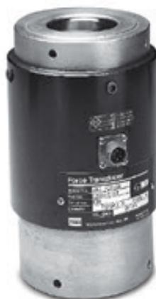
These load cells are fatigue rated.
