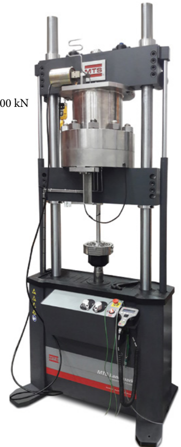
MTS Landmark Test System with Top Industrie Autoclave
