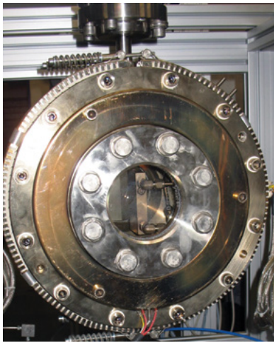
Autoclave with optional optical quality glass window to accommodate non-contacting strain measurement solutions.
