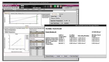
The modulus check confirms the material constant for loading and unloading modulus. Shown here are thermal ramps, modulus measurement, and comparison to known values A results screen confirms the material constant for loading and unloading modulus.
