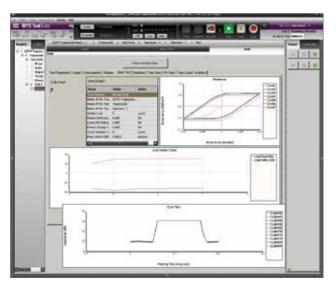
Simultaneously monitor hysteresis loops, load peak and valley per cycle and time trace per cycle in the Runtime View.
