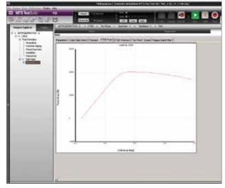
The Runtime View of the pre-crack portion of the CTOD intuitively displays load versus COD.
