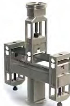
Fully Reversed Loading Double Cantilever Bend Fixtures
