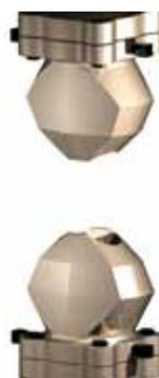
Flat specimen, low-mass tensile grips are specially machined to remove as much extraneous mass as possible.
