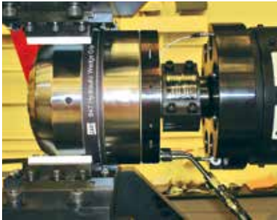
The white polymer pads are part of the passive restraint hardware that protects the load train in the event of specimen failure.
