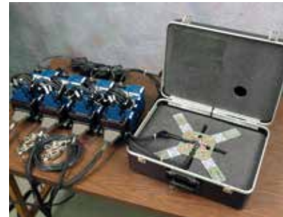
MTS Series 709 Alignment Electronics for conditioning the 32 strain gages mounted on the cruciform alignment specimen.
