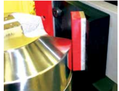
Close-up showing the polymer pads (in this case, red) which restrain the load train components in the event of compressive specimen failure.
