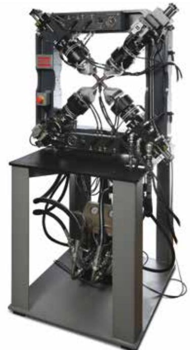
MTS Planar Biaxial 25 kN System designed for mounting on a goniometer for presenting the specimen at variable angles and positions to a high-energy beam for High-Energy Diffraction Microscopy.
