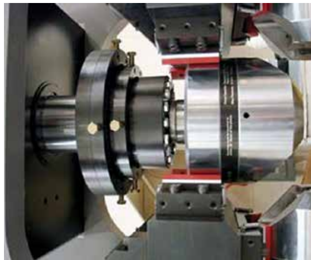
The spherical bearing alignment assembly is to the rear (left) of the grip. The concentricity and angularity adjustment bolts are gold color hex bolts protruding from the containment rings. The red polymer pads are part of the passive restraint hardware that protects the load train in the event of specimen failure.
