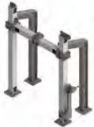
Portal Frame 46.8 kN dynamic max loads (65 kN static) 300-degree Turning Beam width 63 in, max height 74 in
