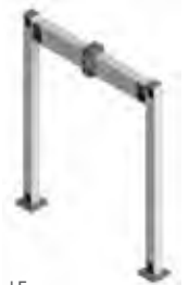
Portal Frame 46.8 kN dynamic max loads (65 kN static) Cross Beam width 82 in, extended max height 104 in
