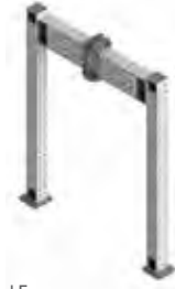
Portal Frame 180 kN dynamic max loads (250 kN static) Cross Beam width 78 in, max height 100 in
