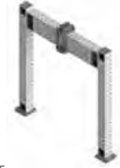
Portal Frame 180 kN dynamic max loads (250 kN static) Cross Beam width 78 in, max height 80 in
