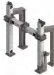
Portal Frame 100 kN dynamic max loads (160 kN static) 300-degree Turning Beam width 65 in, max height 65 in
