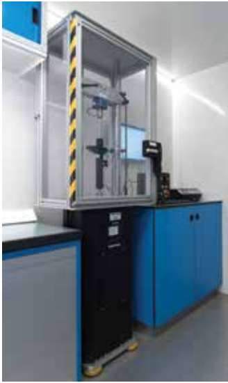
MTS Roehrig EMA damper test system deployed in Tenneco mobile ride tuning truck.
