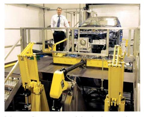
"We're trying to roll as many tests as we can into a single physical prototype," Payne said. "It's more complex, but we're actually saving a great deal of time during development. The test is also more robust because the system interactions are all working together, which is a lot more realistic."
