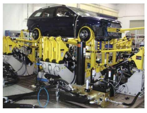
capabilities. It installed several sets of vehicle road simulation test beds, a simulation test platform (MAST), a small 3DOF vibration table composed of various actuator cylinders, a suspension test bed, a steering gear test bed and more. This wide array of equipment has also enabled the PAATC to develop a very well-trained staff of testing technicians.
