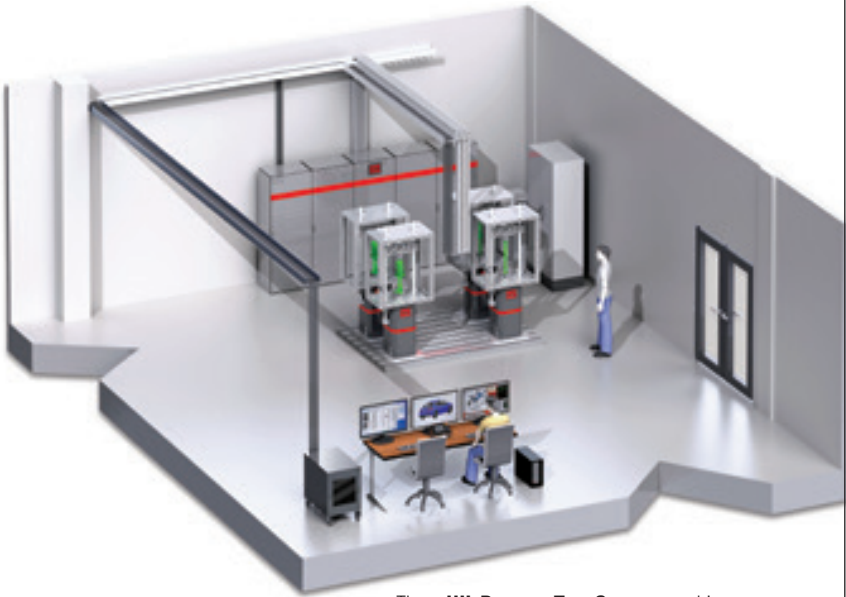
The mHIL Damper Test System combines a physical sub-system of components with a vehicle model adapted for damper and spring inputs.
