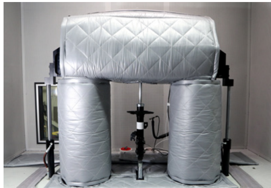
Damper Acoustic Analysis: air-borne “swish” and “squeak”
