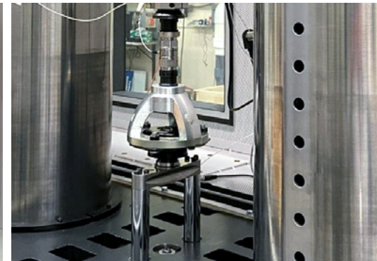
Elastomeric components testing up to 400 Hz
