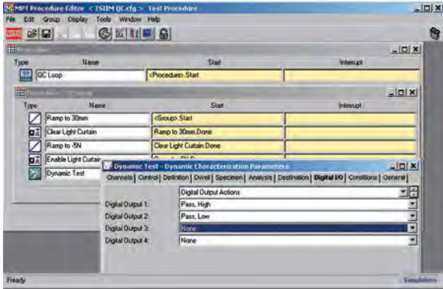
Fig 5. Define the digital outputs for communicating the test results to the external digital devices.
