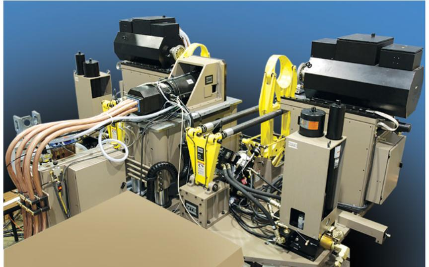
Example of installation for F1 Gearbox testing (with specific high speed input dynamometer)
