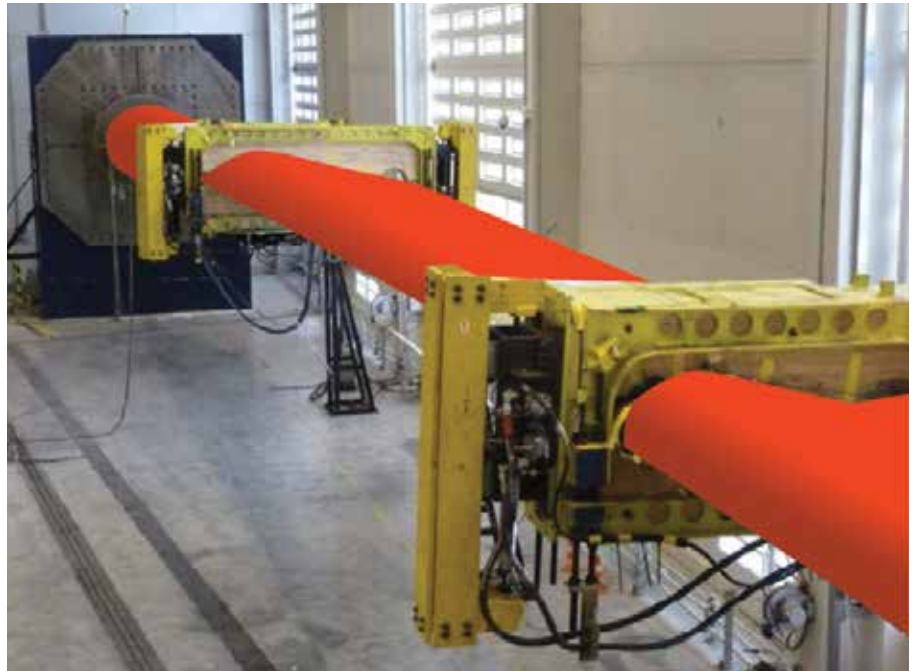
Inertial Resonance Excitation (IREX) Systems deployed for blade fatigue testing (blade visually obscured at customer's request)
