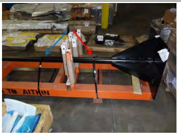
The part was not strapped tightly enough to the metal transfer pallet which can cause the part to fall off and get damaged.
