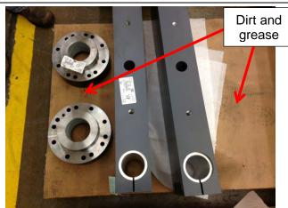
Not enough foam is on the pallet to separate all materials from dirt, grease, and metal shavings present on cardboard.
