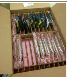
Parts which have been placed in their respective protective wrappings are packed in the manufacturer's box which uses dividers and foam to provide separation and stability.
