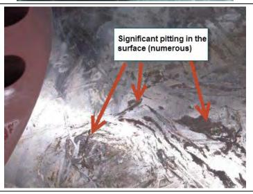
Part was sealed and coated with rust inhibitor to protect it from the environment, but protection was not adequate for longer term storage conditions which allowed rust to form on part.
