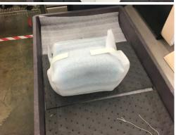
Bare steel is protected with rust inhibitor and then placed in sealable bag to protect it against environmental effects such as rust.
