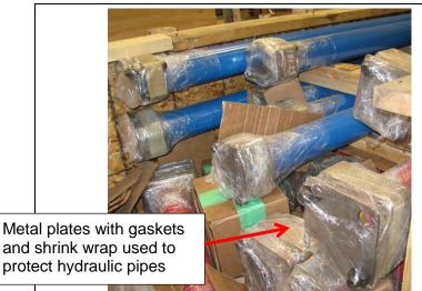
Parts with openings or ports such as pipes, hoses and manifolds need to be sealed well enough to protect against environmental effects and debris which could contaminate systems.
