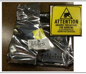
Electrical components which are sensitive to electrostatic are placed in static shielding bags to keep them from being damaged by static discharge.
