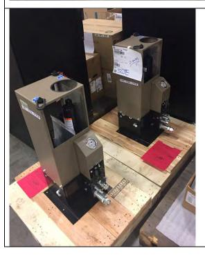
Parts that do not have adequate strapping/bolting could fall over and get damaged or cause injury
