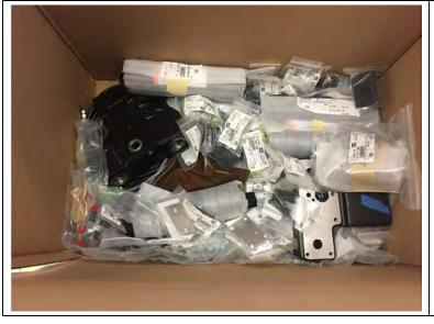
Materials placed in a box with a lack of separation could contact and potentially damage each other.
