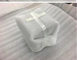
Parts with protective finishes including black oxide, anodized or zinc plated must be placed into sealable bags or wrapped in plastic, creating an environmental seal to protect against dirt, debris and moisture.
