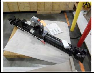
The pallet supporting this part is not correctly sized. The part is hanging off the edges of the pallet and the part is not fully supported or protected.
