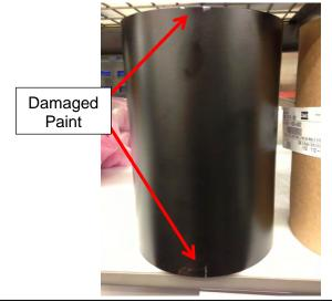
Part was not wrapped and did not have enough protection and separation which allowed the finish to become damaged.
