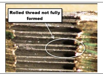
Rolled threads that are not properly formed are unacceptable. This can lead to larger then specified minor diameter, lower thread strength, and could lead to miss-threading the fastener.
