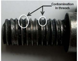
Dirt, grease, chips, and contamination in threads are unacceptable and can lead to poor assembly, contamination of the hydraulic system or improper torque values.
