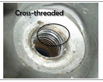
Threads that are cross-threaded are unacceptable. They can prevent future thread engagement and can lead to decreased fastener strength, incorrect torque values and overall unacceptable quality appearance.
