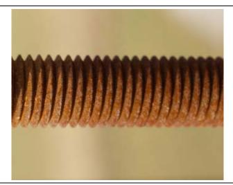
Threads shall be adequately protected to prevent corrosion. Corroded, rusted, or excessively oxidized threads are unacceptable and can lead to decreased fastener strength, incorrect torque values and overall unacceptable quality appearance.
