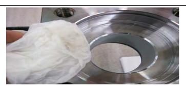
1.4.2 Part is clean and free of cutting fluids, metal chips and debris.
