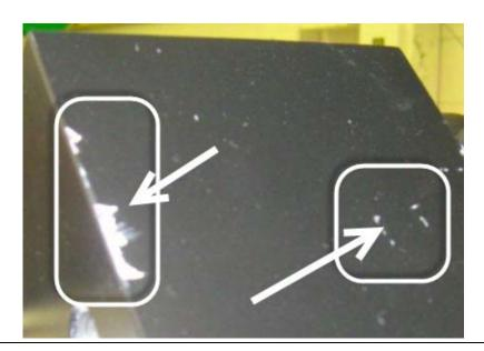
Paint is chipped. This presents an unacceptable appearance. Also, primer and substrate are showing which can lead to corrosion.
