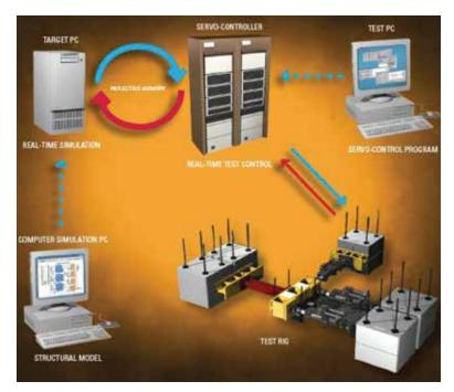
Real-time Hybrid Simulation System Diagram
