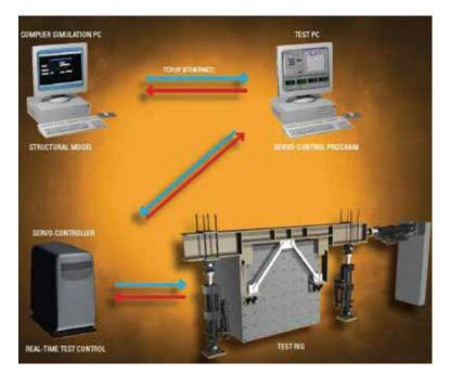
Quasi-static Hybrid Simulation System Diagram
