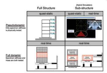
Comparison of Conventional and Hybrid Simulation Testing Techniques
