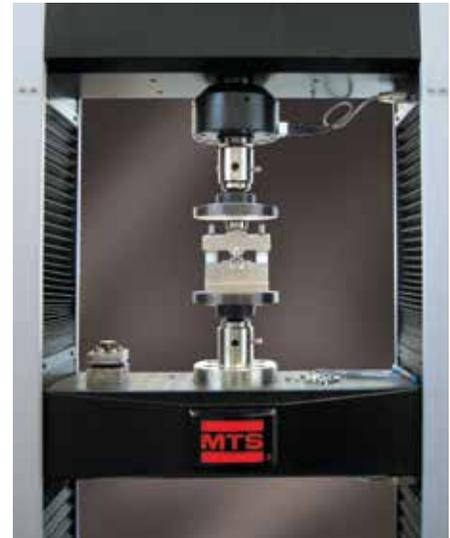
*K4Sint utilizes a unique three-point bend fixture and other fixtures in their MTS Criterion Series 40 Electromechanical Universal Test System to characterize the hardness of new alloys as well as evaluate their yield strength, ultimate tensile strength and ductility.*
