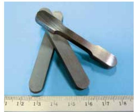
*These metallic bar and dog-bone sample specimens are used to characterize behavior through tensile testing.*
