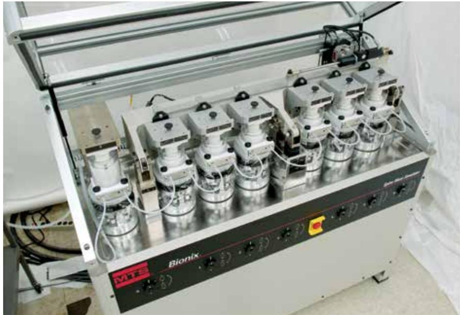
*The Bionix Spine Wear Simulator features six active specimen containment modules to provide a statistically valid sample size.*
