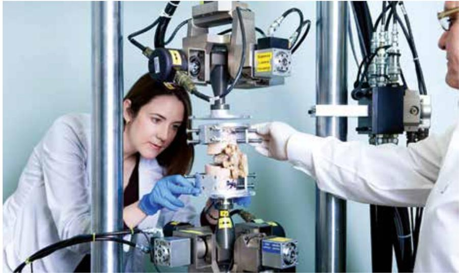
different designs of posterior dynamic stabilization devices for the lumbar spine. Recently, the researchers have been evaluating different surgical techniques for correcting spine deformity in adolescents, a complex biomechanical problem.
