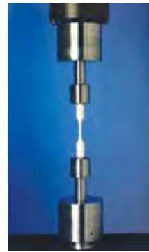
Bionix accessories include grips, fixtures, platens and baths for a diverse range of biomedical specimens.
