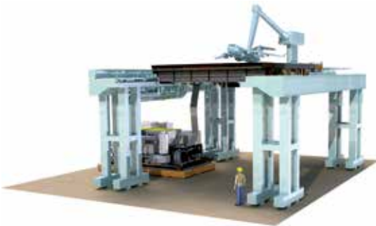
DNW's wind tunnel rolling road provides the most realistic simulations possible for manufacturers who seek to perform complete aerodynamic optimization of new aircraft, as well as upgrades for existing aircraft.
