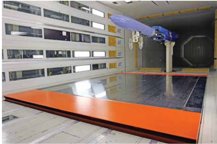
The speed, flatness and reliability of DNW's MTS wind tunnel rolling road system enables manufacturers to accurately and efficiently replicate the unique dynamics surrounding aircraft takeoffs and landings
