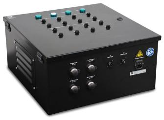
AC&A signal hubs provide 24V power to AC&A valve isolation solenoids and electronics, and have the capacity to control up to 8 valves/channels per hub. Compact AC&A signal hubs can be located around the test article, minimizing the cabling needed to reach actuator-mounted valves/manifolds. Integrated health monitoring provides real-time valve diagnostics and fault detection, and an uninterruptable power supply (UPS) ensures safe unloading even during total power failure.
