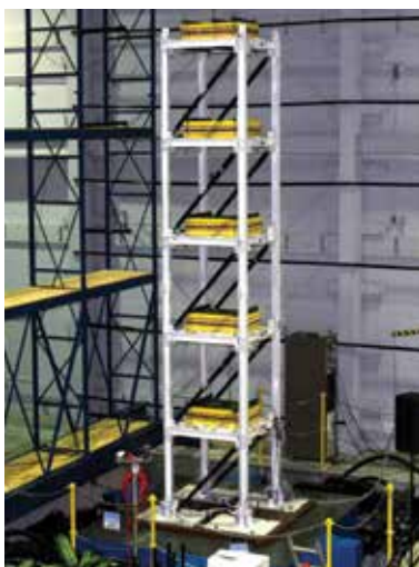
Testing of added clamping system in 5-story structure
