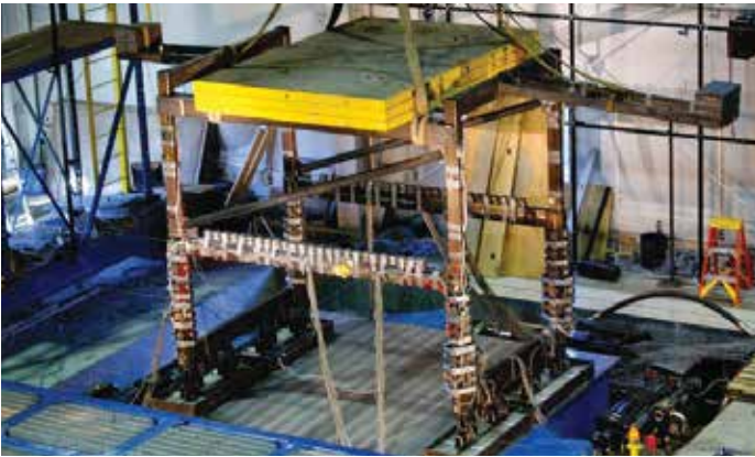
Large-scale, shake table test of container crane
