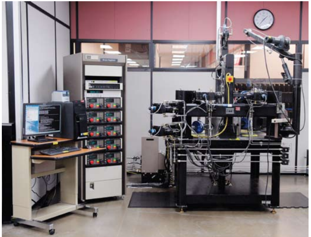
SWIFT transducer calibration stand
