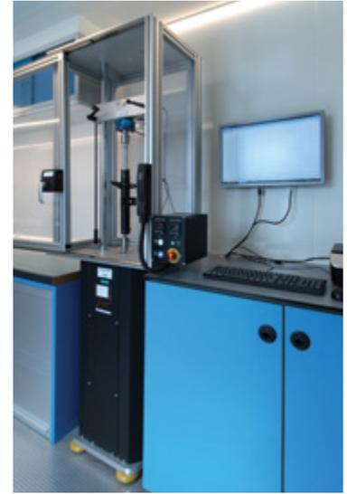
MTS Roehrig EMA damper test system deployed in Tenneco mobile ride tuning truck.
