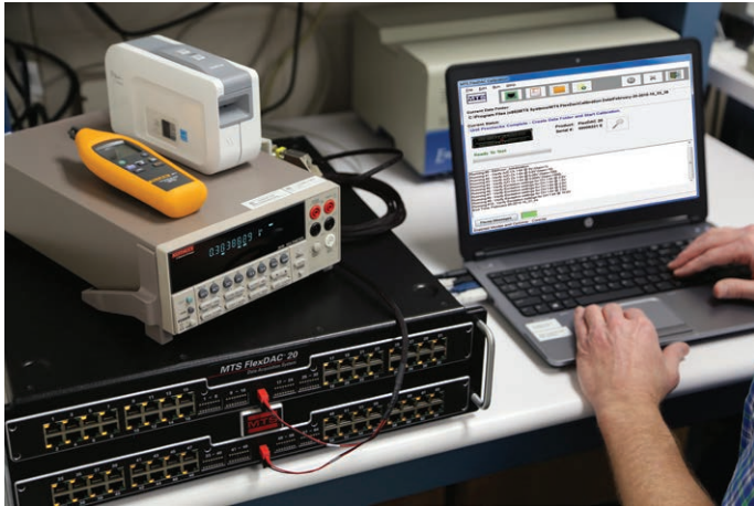
The Calibration Kit includes a laptop, multimeter, temperature/humidity meter, label printer and cables
