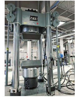
A high-force, floor-standing MTS load frame provides component and materials testing capabilities
