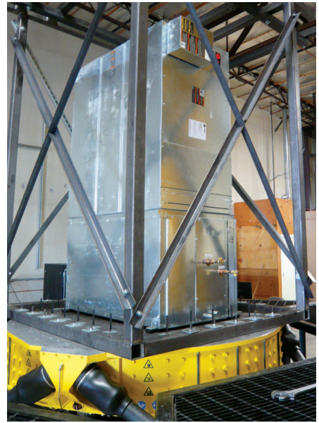
The MTS 353.20 MAST™ system proved instrumental in helping DCL quickly establish OSHPD certification testing capabilities
