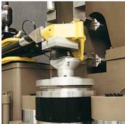
crosshead for easy specimen mounting and ready access to test space. Large diameter, hollow columns and a light but stiff crosshead load unit provide more accurate displacement measurement than other designs. Another attribute is the fact that the load frame resonance is outside of the operating frequency range, providing better phase, load, and displacement resolution within the system's wide operating range. Strut and flexure assemblies
