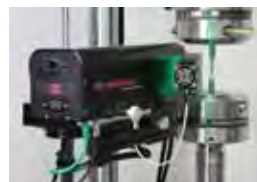
Non-contacting Optical & Video Extensometer for Tension, Tensile Shear, Fatigue & Fracture Testing
