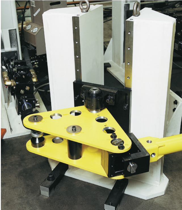
Reaction stands shown with a bell crank
