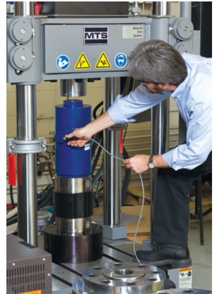
Load Frame Calibration
