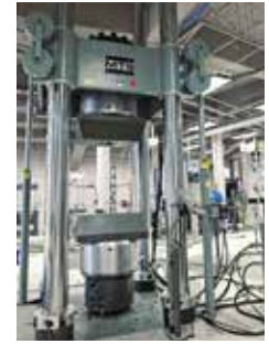
A high-force, floor-standing MTS load frame provides component and materials testing capabilities
