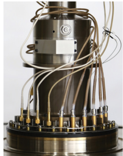
The Ultrasonic Velocity triaxial platens propagate a compression wave and two orthogonal shear waves along the longitudinal axis of the core sample. The system then measures the time of flight through the specimen, calculating dynamic elastic properties that can be compared to static properties collected using traditional techniques.
